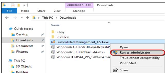
Figure 6: The **Run As Administrator** command is in the right-click submenu.
