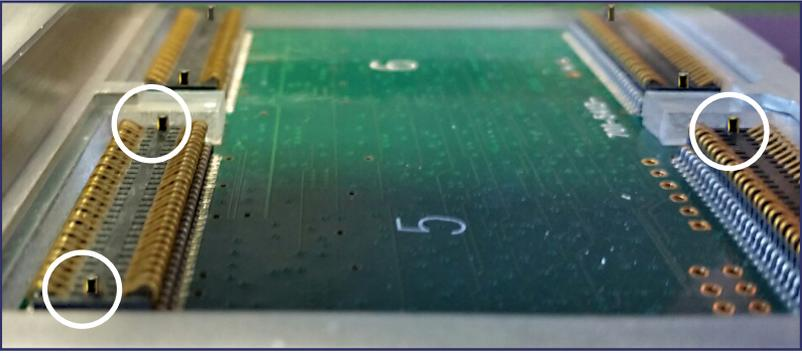
Figure 3: Alignment pins (three of the four shown, circled).
