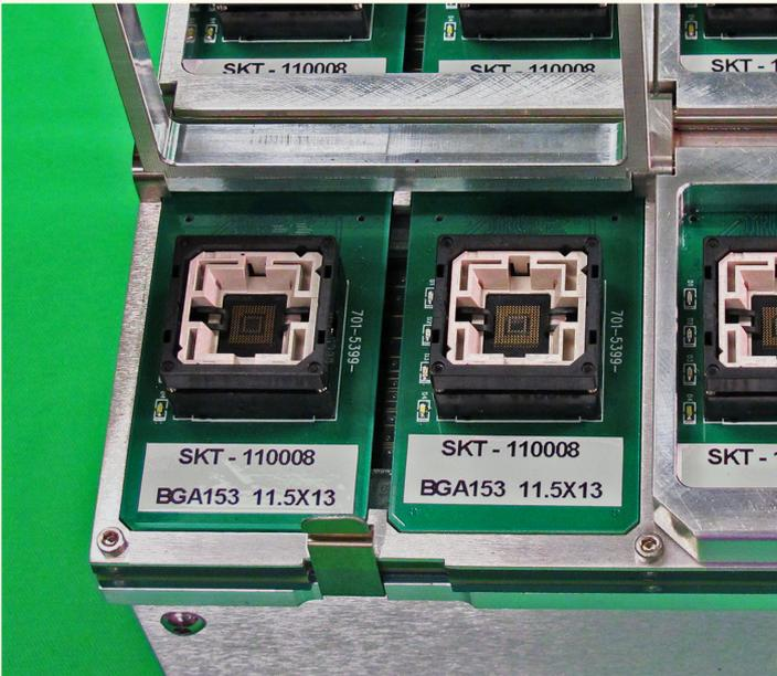
Figure 4: Note chamfered (angled) corners on Socket Adapters fit into programmer body. (One clamp is open.)
